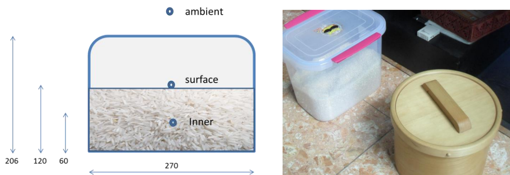
Figure 6. Relative humidity: (a) measurement setup, (b) comparing plastic and wood barrel.
