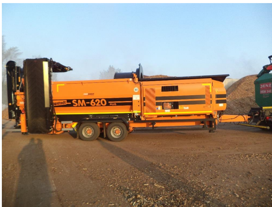
Figure 6. Doppstadt SM 620 plus type mobile star riddle (Photo F Szűcs).
