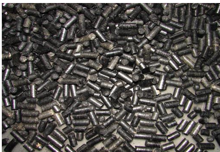
Figure 2. Carbon black 5% and pine shaving 95% blend pellets.
