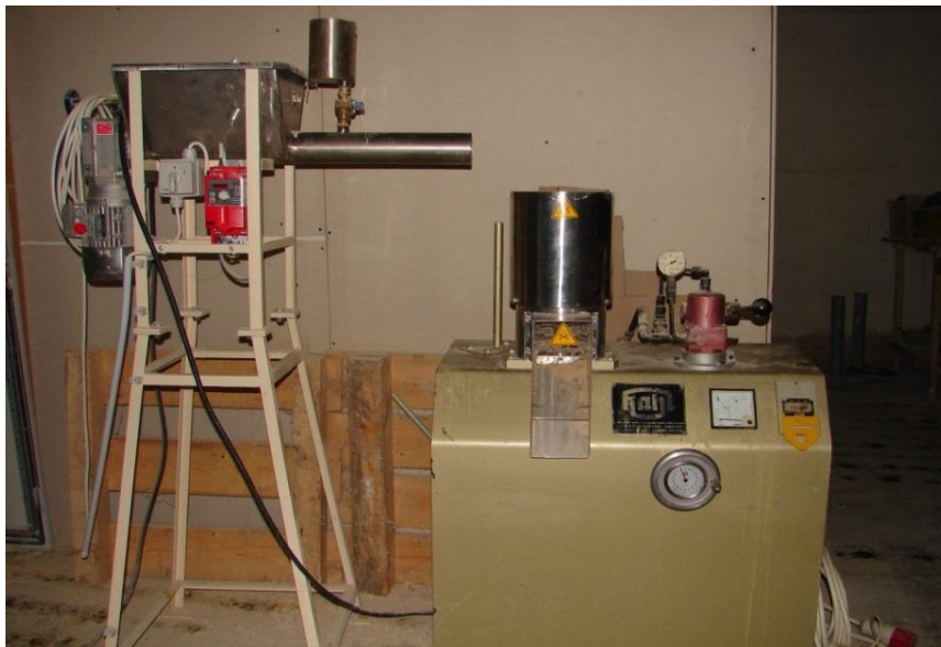
Figure 1. Kahl type pellet press with feeder.
