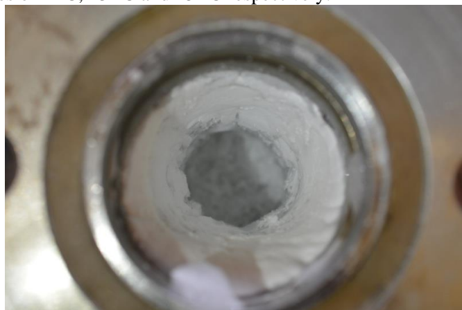
Figure 4. The image of 500 ml reactor with methane hydrate obtained from 100\text{ cm}^3 aqueous SDS solution (0.1%).
