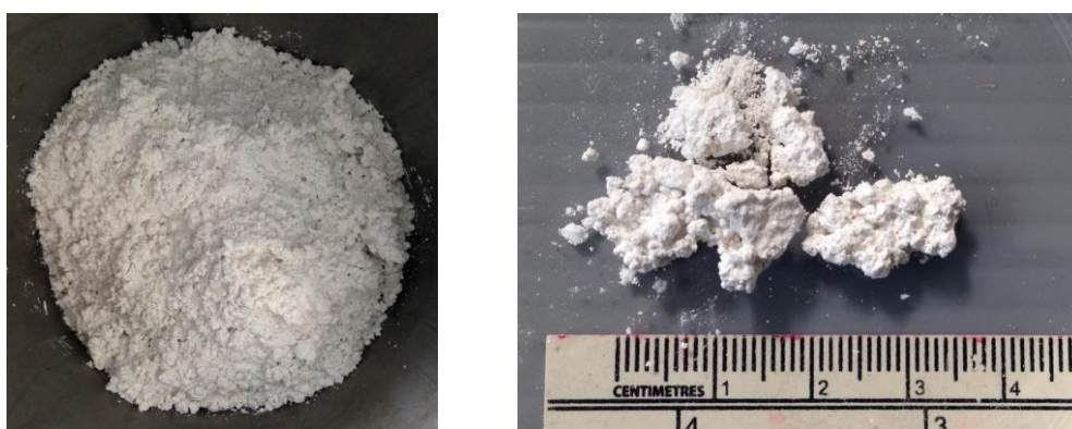
Figure 6. Agglomeration of powders in the reactor after hydration reaction.
