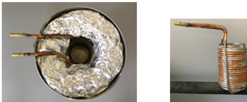
Figure 4. Reactor and heat exchanger arrangement.
