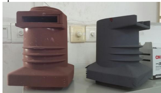
Figure 1. After coated, the coating fell off.
