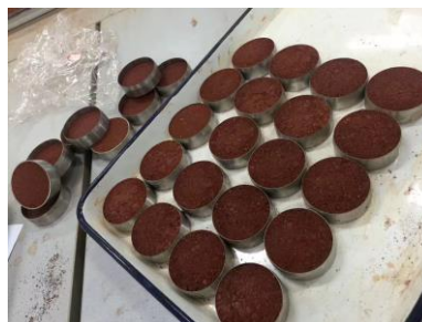
Fig.1 the laterite sample used for direct shear strength
