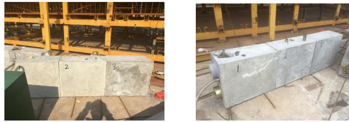
(a) Test specimen of group A (b) Test specimen of group B Fig.3 leakage test of sealing device
