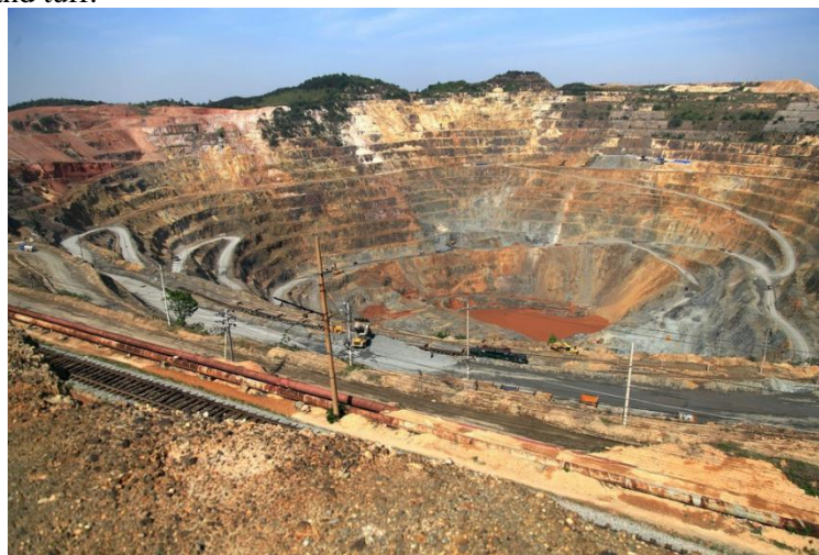
Figure 1. Washan deep concave type iron ore stope
