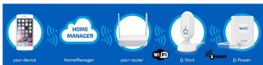
Figure 3. How NorthQ Electricity Starter Kit Works
