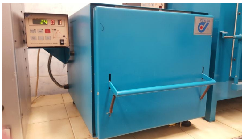
Figure 1. Muffle furnace produced by Czylok-Sel
