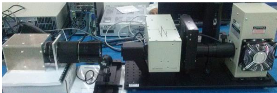
Figure 2. Test with monochromator.
