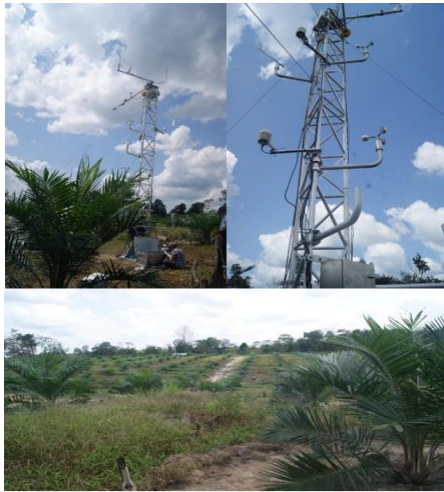
Figure 2. Research site in Pompa Air Village with micrometeorology tower installed on a 2.5 years old oil palm.
