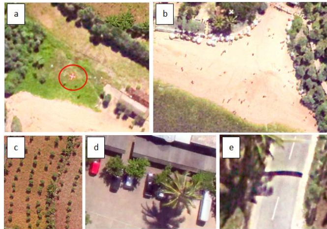
Figure 5. (a) The visible pre-mark, (b) the recognizable distribution of tourists on a sandy beach, (c) the visible individual stand of cassava, (d) the size and type of cars identified from aerial photos, and (e) apparent road markings.
