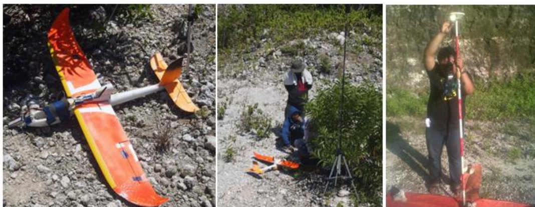
Figure 3. (a) Bixler, the UAV Used for Photography, (b) Preparation, UAV component Setting, and Ground Control Station, (c) Pre-mark Installation and Ground Control Point Measurement by Team Member During Preparation.
