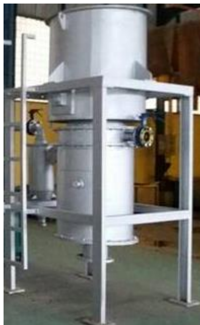
Figure 3a. Gasifier type downdraft designed and used in this research
