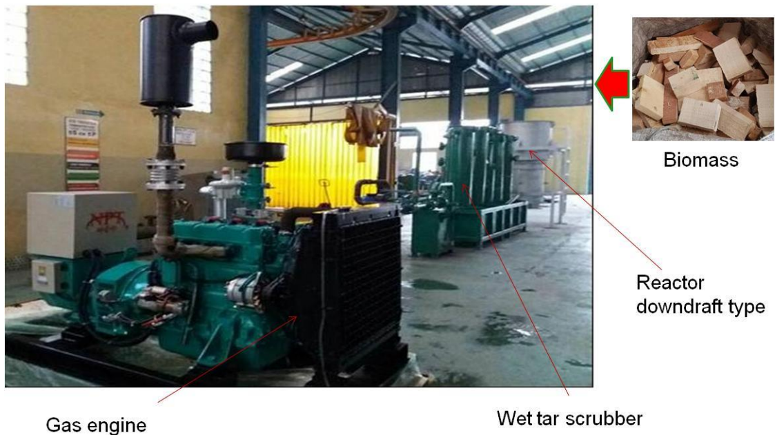
Figure 4. Biomass Power Generation with Capacity of 25 kW
