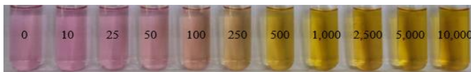
Figure 5. Color sensitivity of purple sweet potato's anthocyanin against sodium nitrite in various concentrations (ppm)
