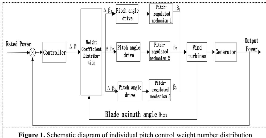
**Figure 1.** Schematic diagram of individual pitch control weight number distribution
