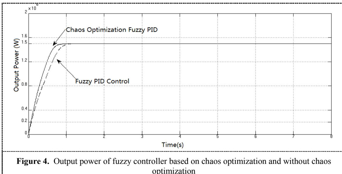
Figure.4 shows the output power simulation of fuzzy PID control which has been Chaos optimized and not optimized. The simulation results show that under the same conditions, the fuzzy PID controller optimized by chaos algorithm controls better and faster than the one without optimized.
