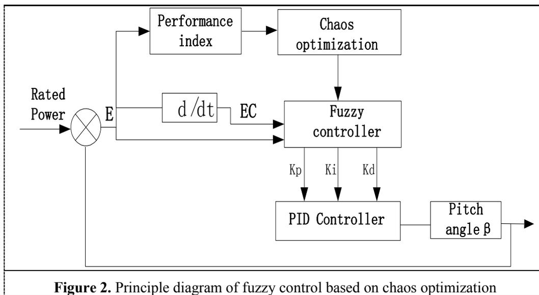
**Figure 2.** Principle diagram of fuzzy control based on chaos optimization
