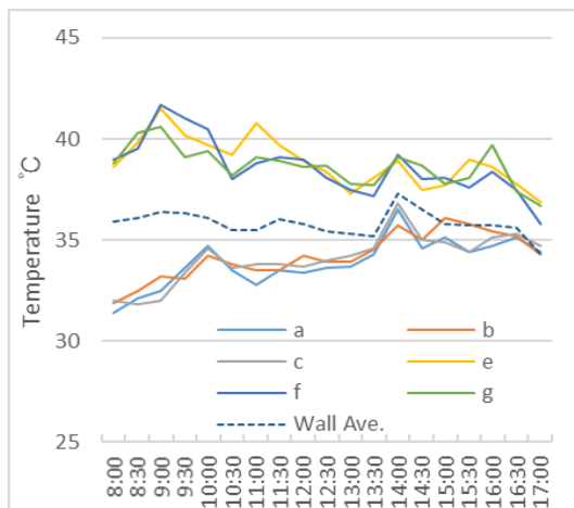
Figure 14. Surface Temp of GF A (a-c: GF; d-e: the bare wall; Wall Ave.: the whole wall Ave. Temp; 8/8/2017 8:00-17:00)
