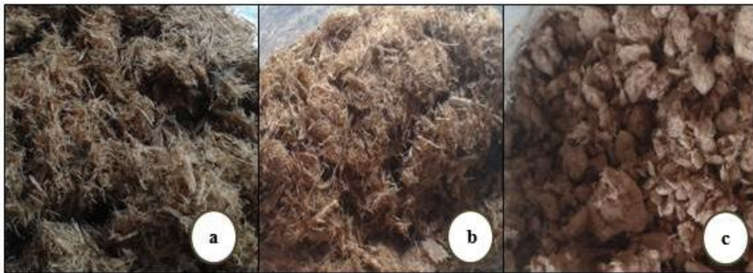
Figure 2. Pulp properties (a) 2% NaOH (b) 4% NaOH (c) 6% NaOH
