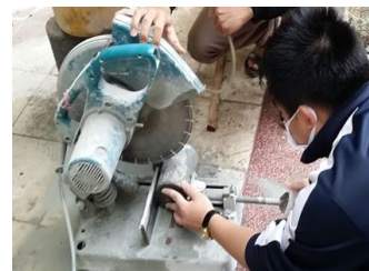
Figure 5. Cut cylindrical concrete sample of 5x10cm.
