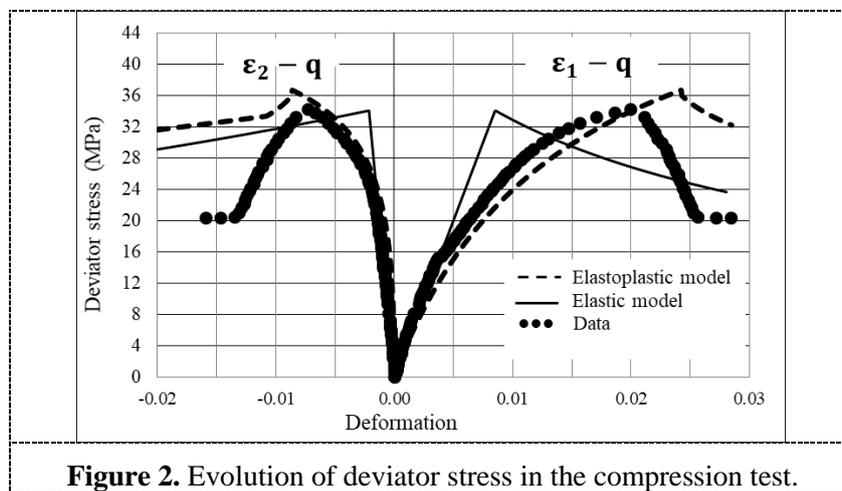
**Figure 2.** Evolution of deviator stress in the compression test.
