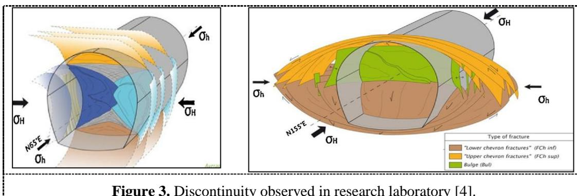
**Figure 3.** Discontinuity observed in research laboratory [4].
