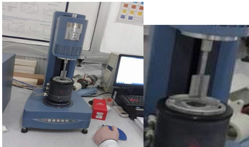
Figure 2 : Rheometer AR2000 used for rheological study.
