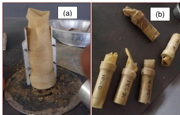
Figure 1. (a) Preparation of compacted specimen, (b) Marked specimens.
