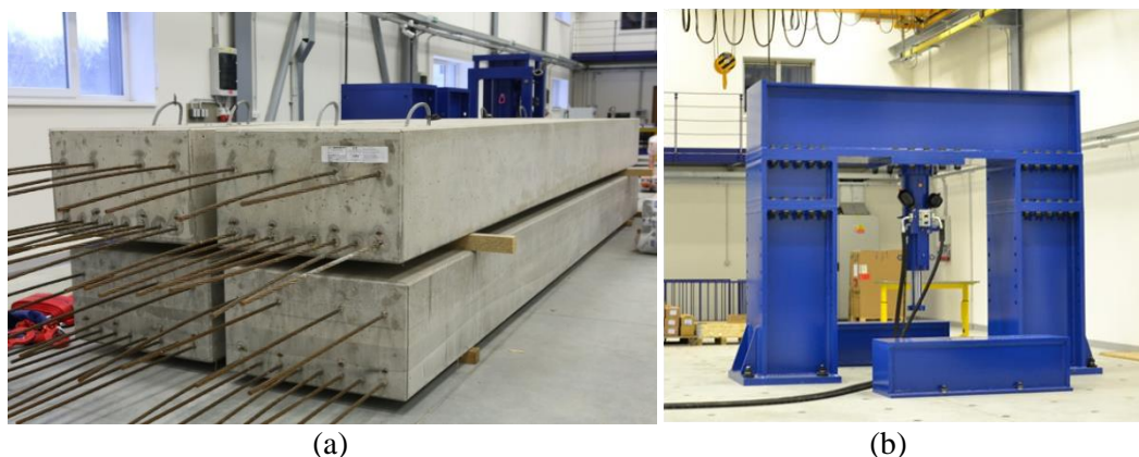
Figure 1. Preparation of laboratory evaluation of carrying capacity: (a) Samples of prestressed concrete beams and (b) Test machine pressing head.
