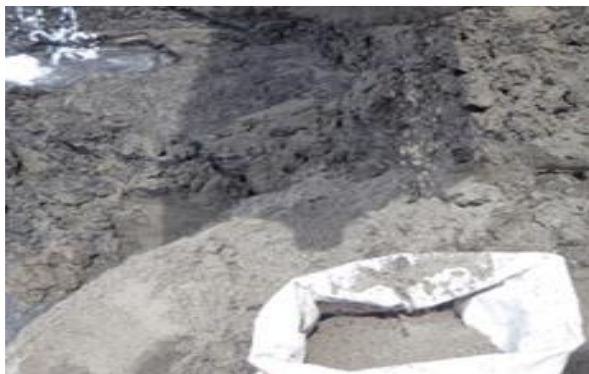
Figure 1. Palm oil fuel ash is packed in gunny sack
