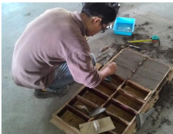
Figure 5. Casting of brick specimen
