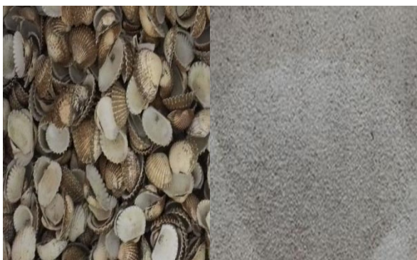
Figure 4. Cockle shell before and after processing
