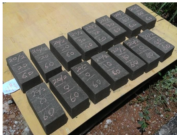
Figure 6. Brick samples ready to be water cured
