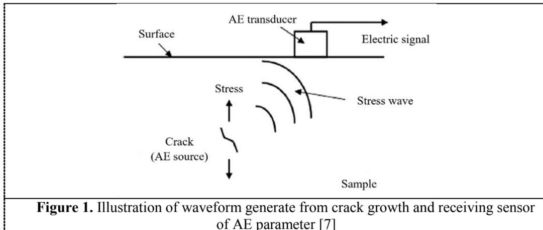
**Figure 1.** Illustration of waveform generate from crack growth and receiving sensor of AE parameter [7]
