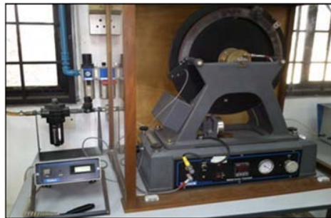
Figure 3. Rebound resilience test machine
