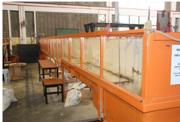
Figure 2. A 11 m long \times 0.6 m deep \times 0.5 m wide flume
