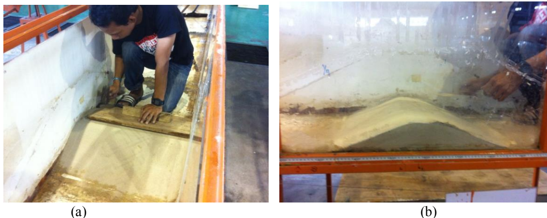
Figure 3. Compacting the embankment; (a) compaction method, (b) final shape of the embankment
