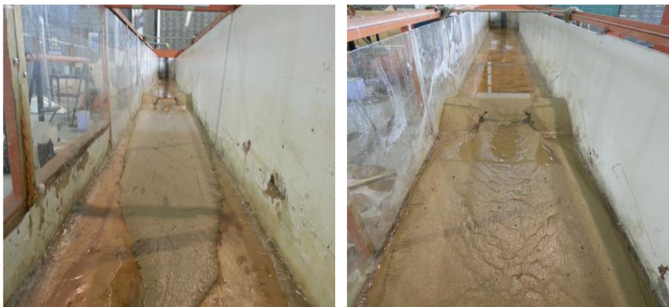
Figure 6. Failure and sediment pattern at downstream after completely breached
