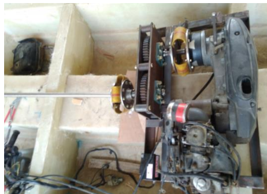
Figure 3. Setting the motor engine as catamaran motor boat driving force.
