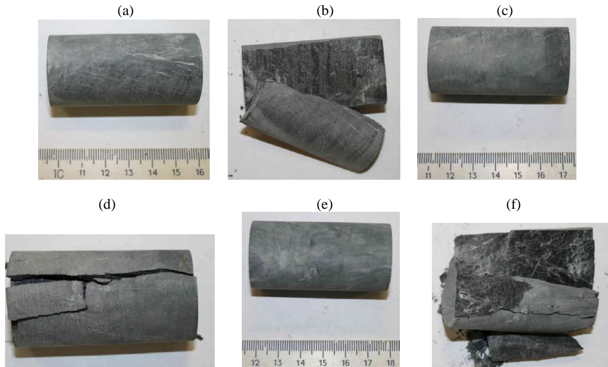
Figure 1. Meta-siltstone specimens (dimension group 1) before (a, c, e) and after (b, d, f) uniaxial compression tests.
