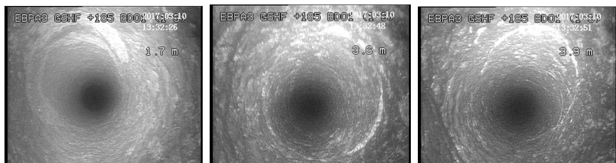
Figure 4. Images of holes and cracks in fan 1.
