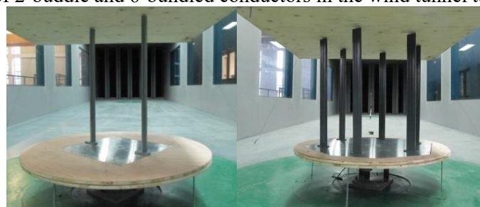
(a) 2-bundled Conductor Model (b) 6-bundled Conductor Model
