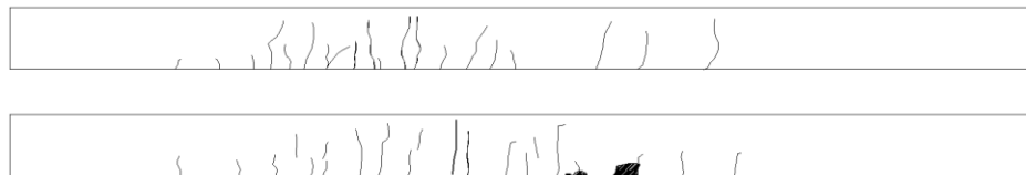
Figure 4b. Crack distribution at the two lateral surfaces of Plate A.
