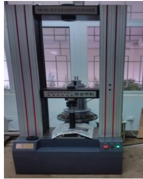
Fig.1 TAW - 200 electronic multi-function material mechanics testing machine
