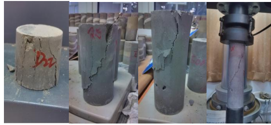
Fig.7 The failure form of different aspect ratio specimen
