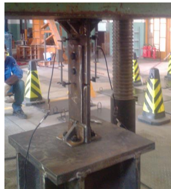
Figure 4. Guide rod extensometer arrangement figure
