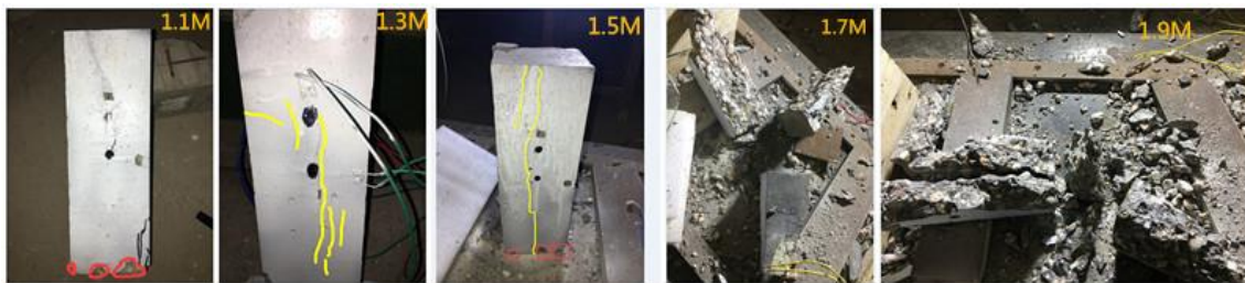
Figure7. Failure mode of specimen under different working conditions.
