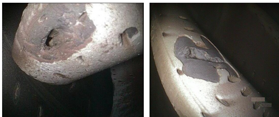
Figure 2. CFM56-7B Engine HPT Defect.
