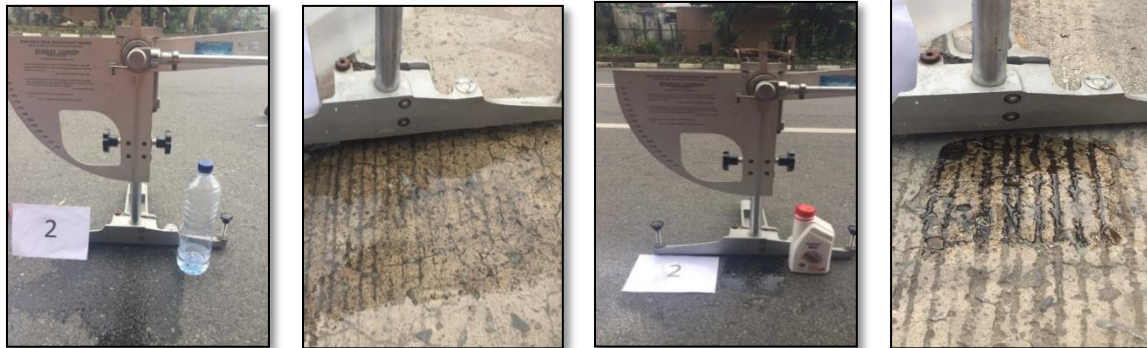
Figure 3. Pavement surfaces affected by water and lubricating oil contaminants
