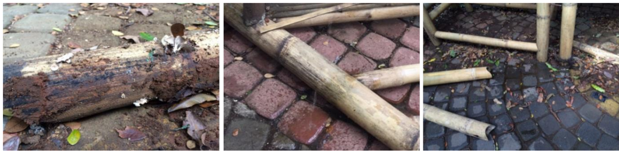
Figure 6. Damage on the bamboo sticks caused by the weather and humidity on the surface of the ground.
