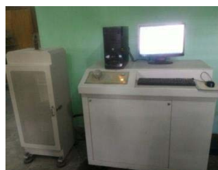
Figure 2. Compression Test Machine GOTech U60
