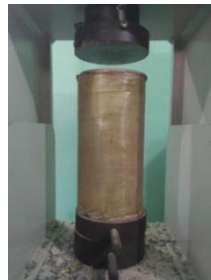
Figure 4. Test Object in Compression Machine
