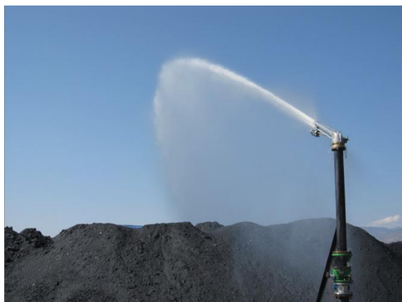
Water mist spraying dustfall
