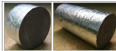
Figure 3. The specimens partially sealed by aluminum foil.
