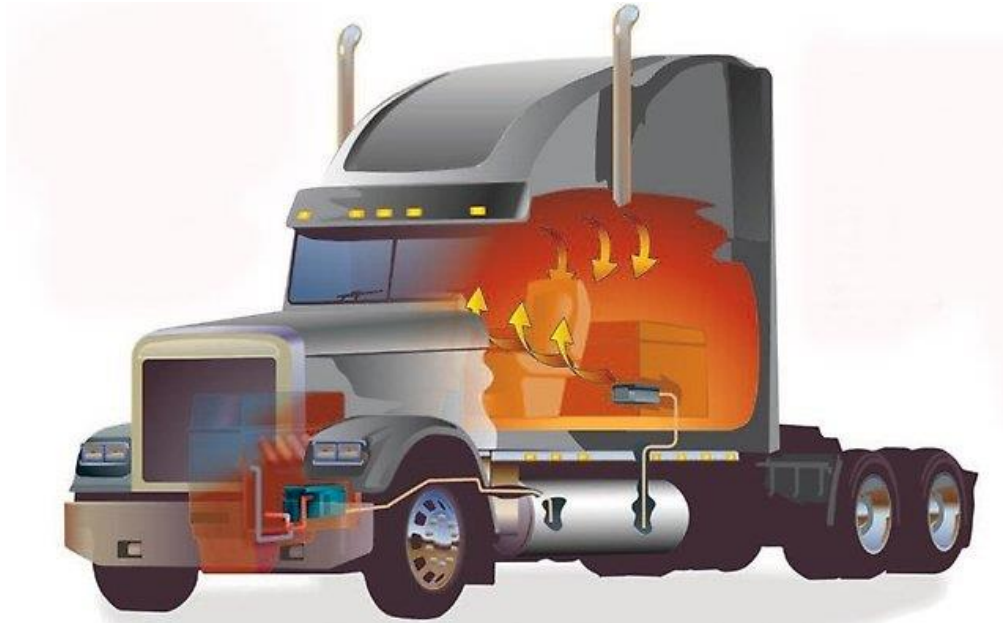
Figure 3. The principle of the self-powered heater operation
