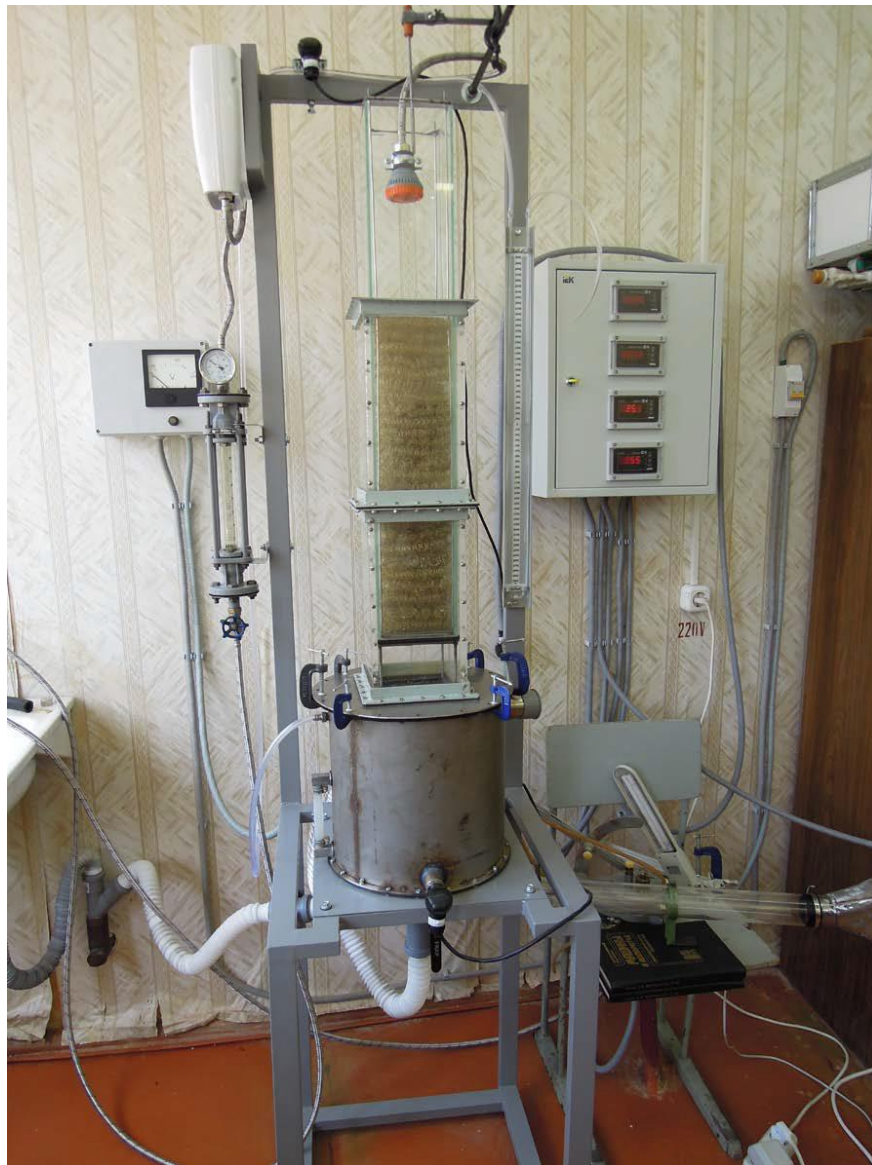
Figure 3. Photo of the experimental setup for the study of hydrodynamics and heat and mass exchange processes in packed devices.
