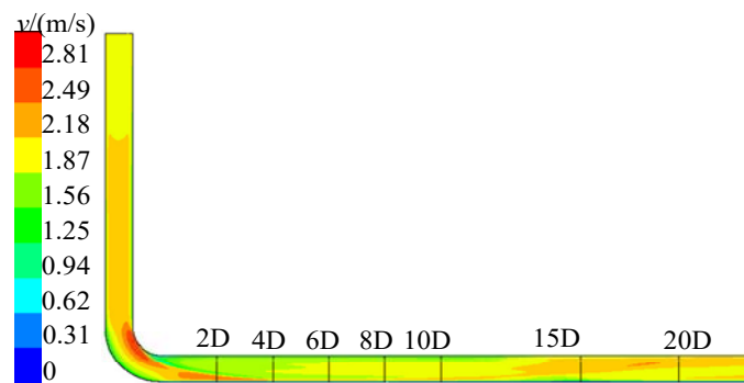
Figure 5. The longitudinal section velocity contour of the pipe with pipe diameter 377mm
