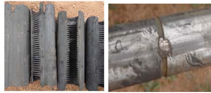
Fig.3 Sucker rod joint with eccentric wear and stuck pump caused by iron filings
