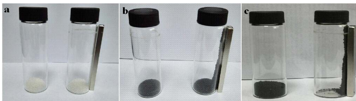
Figure 5. Magnetic adsorption test of (a) pure PMMA (b) PMMA/ 1.0% \text{Fe}_3\text{O}_4 microspheres (c) PMMA/ 2.0% \text{Fe}_3\text{O}_4 microspheres
