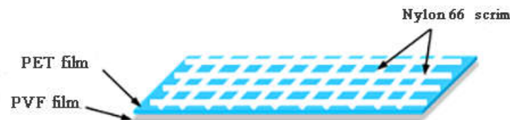
Figure 1. Schematic diagram of nylon 66 scrim reinforced PVF laminated membrane
