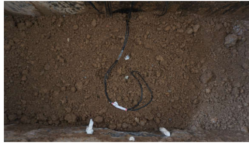
Figure 5. Imbedded grouting rock pressure sensors
