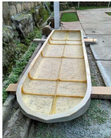
Figure 2. Scaled SPB Model at 2 m Length
